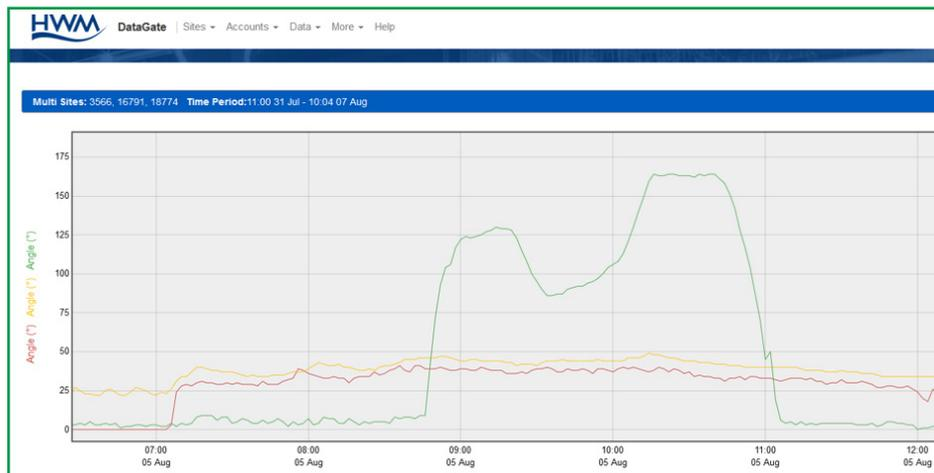
The system is up-to-date too. SpillSens devices call in, at minimum, once a day, whilst also providing alarms when a pre-determined angle is reached.
