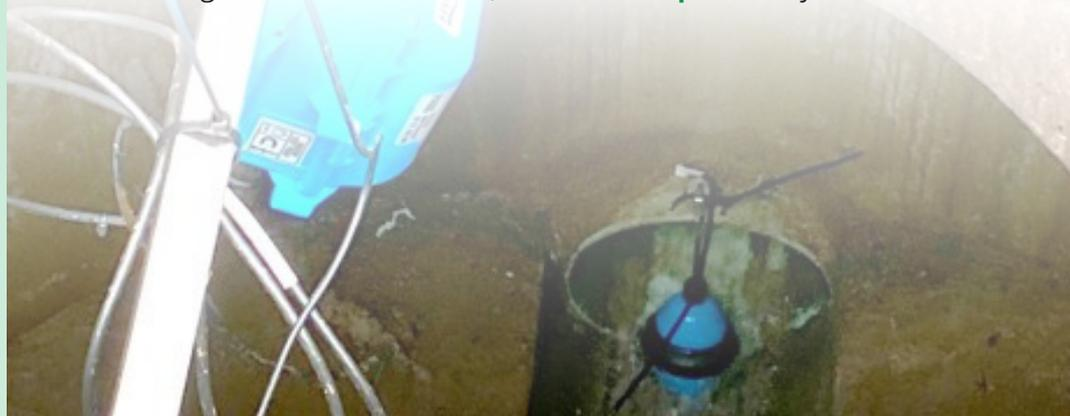
By hanging the angle-based sensor inside the chamber at 'low-flow' level, the authority can quickly track the rise and fall of sewage flowing through the pipe, and compare it with rainfall events to establish the I&I entry points in their system. Analysis of this is simple and clear – the larger the peak during rainfall, the more rainwater is entering the system. The same data can also be used to inform better allocated deployment of inspection equipment, and longer-term system upgrades.
