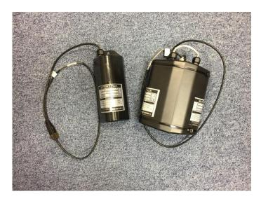
Important: When placing the battery in the site, ensure that it is not crushing any cables other parts of the installation as they are heavy devices. Also respect any orientation arrows on the pack to optimise battery life.
