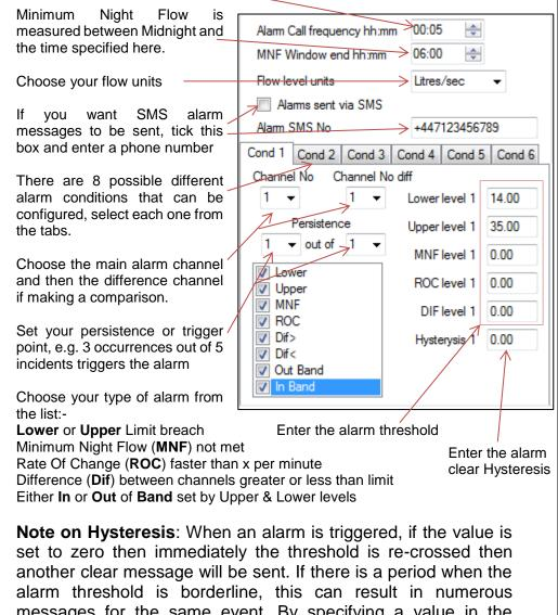
alarm threshold is borderline, this can result in numerous messages for the same event. By specifying a value in the Hysteresis box, you can provide a window that allows the threshold to be repeatedly crossed without sending repeated messages. e.g with an Upper limit of 5 and a hysteresis of 1, the alarm will trigger at 5, but the clear message will not be sent until the value drops to below 4.
