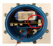
2. Lift out the battery to allow easier access to the SIM card slot
