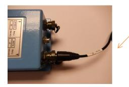
When making a connection to Multilog 2 you will normally need to splice the bare tails together. It is important that a waterproof connector housing is used, such as the "Tuff-Splice" enclosure available from HWM.
