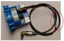
Connect the Plug to the EXT. PRESS socket on the logger. Ensure you feel the 'Click' as the connector locks into place.
