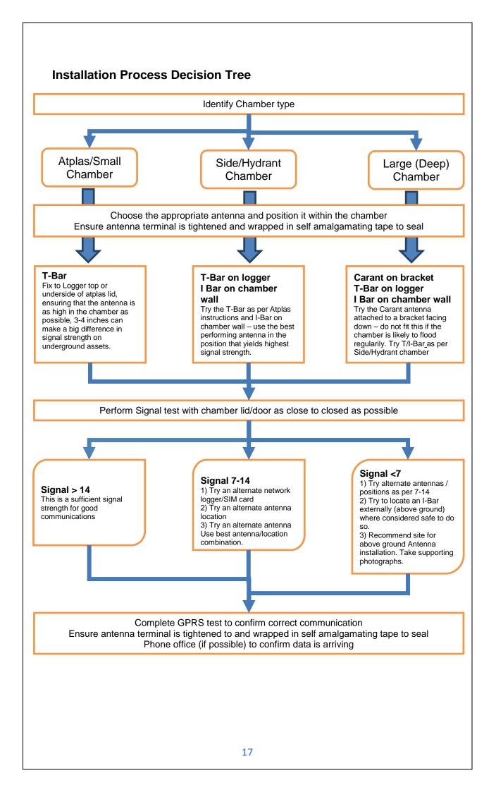
Cellular Network Signal Strength (as measured by CSQ Test)
