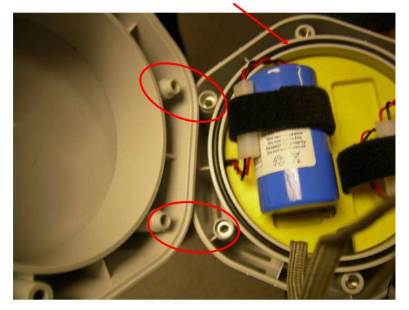
Tighten the lid securing screws to 0.5Nm
