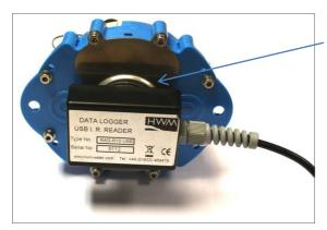
Take care to position the head over raised ring area around the window. The reader head will hold onto the logger by magnets in the ring around the window and this helps with positioning.
