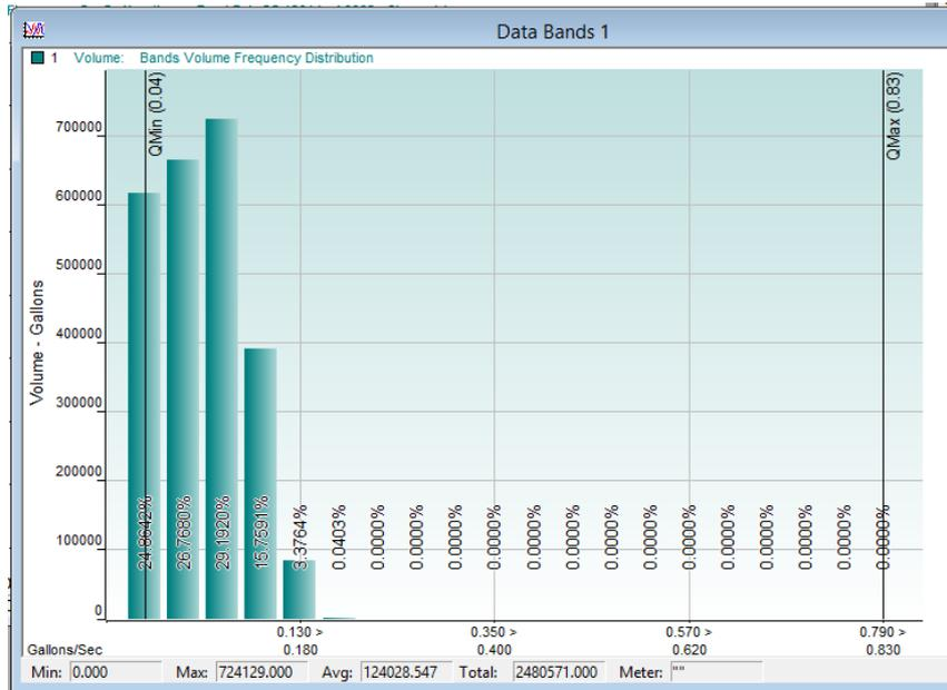
The data bands graph will help you to determine the size of meter required as you would be looking to contain the major flow between the QMIN / QMAX values.
