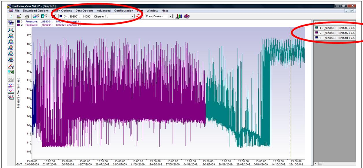
Text can be added to the graph by selecting Graph options, Enter Text – Logger Serial # could be added as shown – it can be positioned anywhere on the graph
