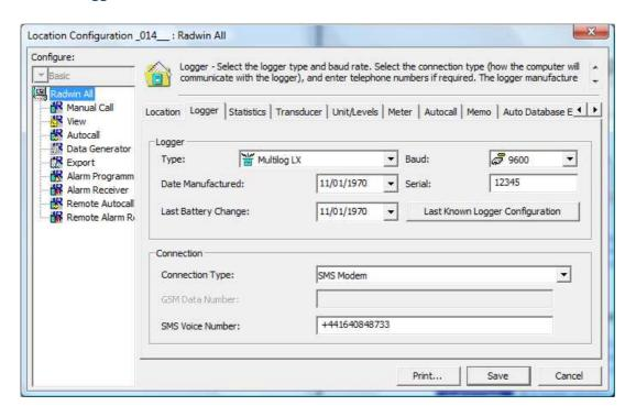
Fill in the logger details as accurately as possible. Logger type from the drop down Baud is automatically filled from the logger type selected above
