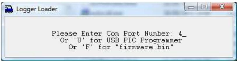
Enter Com port number then ‘Enter’ to reveal screen below - find the first piece of firmware (Hex file) and select it, then select the ‘Open’ button at the bottom of the screen (Note the firmware versions shown here are for illustrative purposes only and are not the ones you require for SoundSens)
