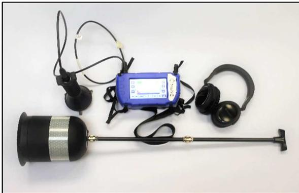
DXmic with optional hand probe and tripod
