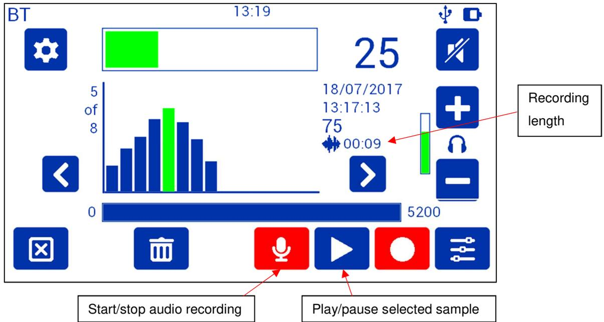
DXmic Pro allows the user to record sound samples when in MLP mode. To start an audio sample recording press the red microphone button. Up to two minutes of sound can be recorded per sample. The recording can be stopped by pressing the stop button, noise level information will be stored with it. The audio recording will appear as a bar in the graph. When a measurement with an audio recording is selected from the graph the recording length will appear under the noise level indicator.
