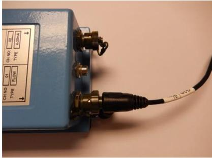
When making a connection to Multilog 2 you will normally need to splice the bare tails together. It is important that a waterproof connector housing is used, such as the “Tuff-Splice” enclosure available from HWM.
