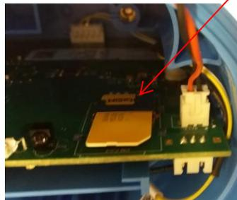
3. Insert your new SIM into the empty slot as shown above. Ensure the gold contacts face the board and the notch is to the left.
