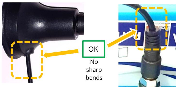
Figure 22. Protect from sharp bends (especially near connectors)
