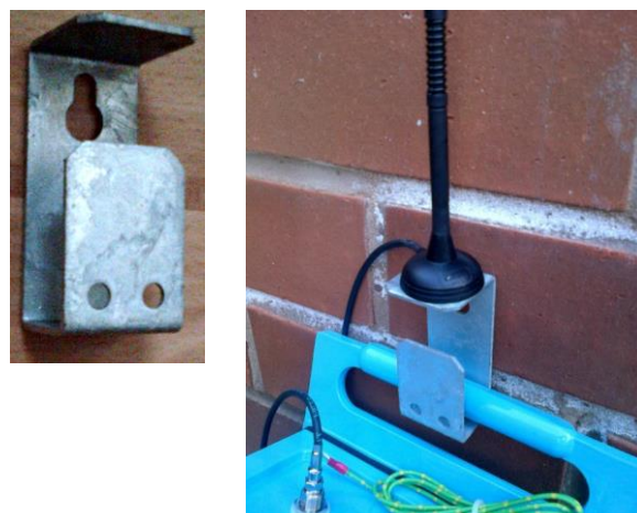
Figure 10. Example installation of Multilog2 using a suitable wall-mount bracket.
