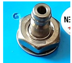
Figure 10. Connection to an internal water pressure transducer
