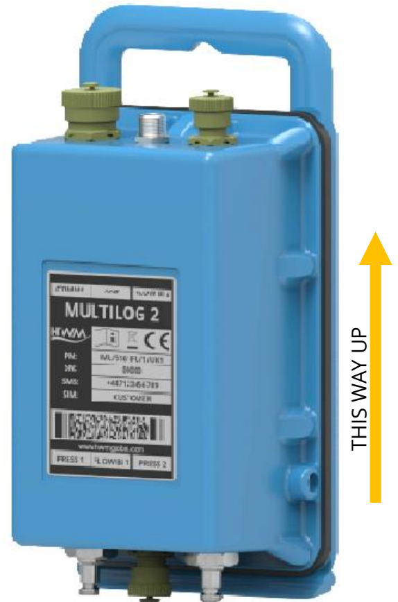
Figure 1. An example Multilog2 Logger. Shows correct orientation for best battery life.
