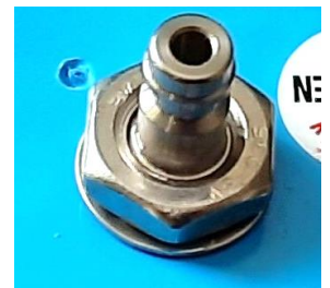
Figure 10. Connection to an internal water pressure transducer
