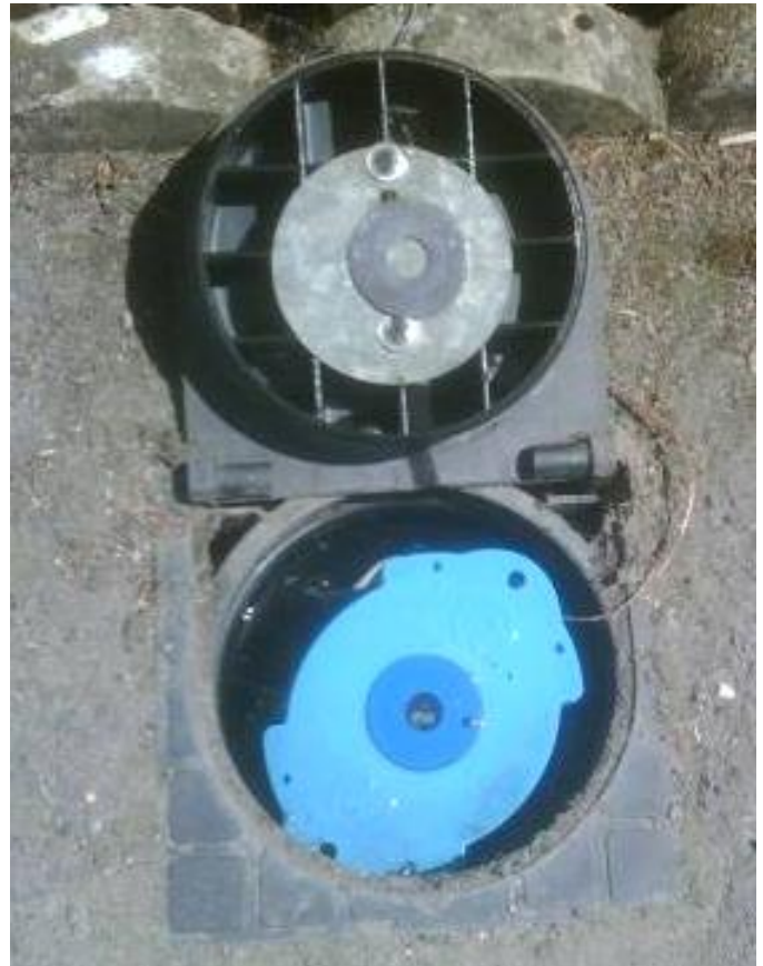
Figure 17. Logger mount using a plastic tube example
