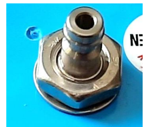
Figure 12. Connection to an internal water pressure transducer
