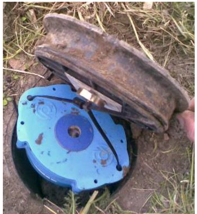
Figure 16. Logger in Talbot flip-lid box P-clip example
