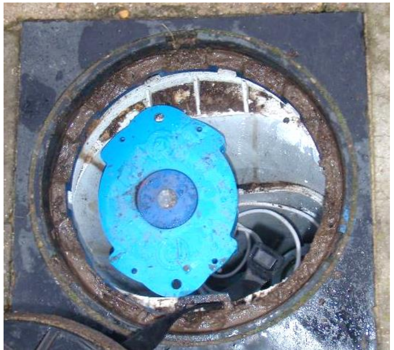
Figure 15. Logger in Talbot round lid box example
