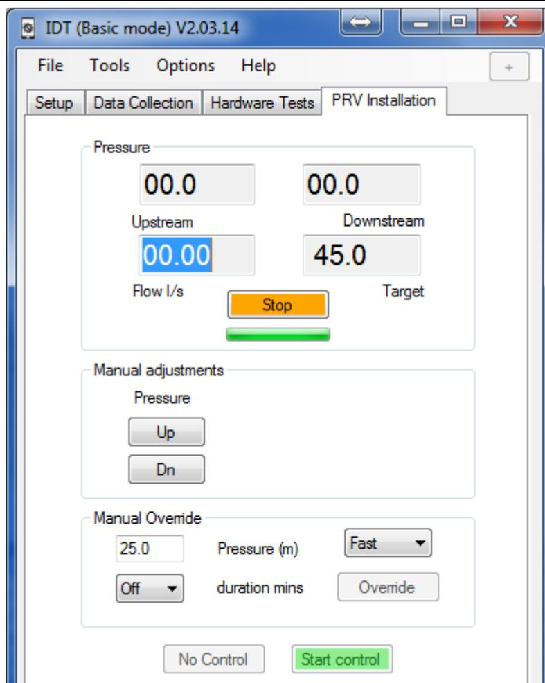
29) Click 'Stop' to come out of 'Live Values' and do a manual override to check that the controller is working or the actuator settings.
