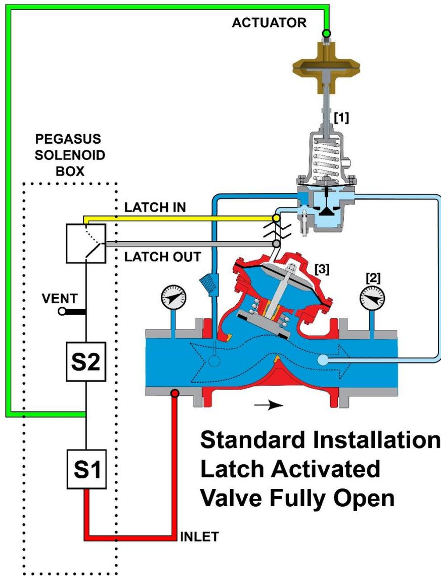
If the Latch is activated, water pressure in the top chamber of the main valve [3] vents to atmosphere and empties, allowing the main valve to fully open.
