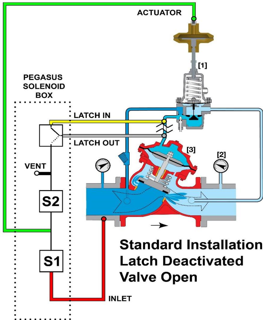
In the above configuration, the upstream water is connected to the Pressure Reducing Pilot [1]. The Latch is deactivated, connecting the pilot to the top chamber of the main valve [3]. The actuator is adjusting the spring in the pilot and therefore adjusting the pressure in the top chamber of the main valve [3], thus controlling how much the main valve opens.
