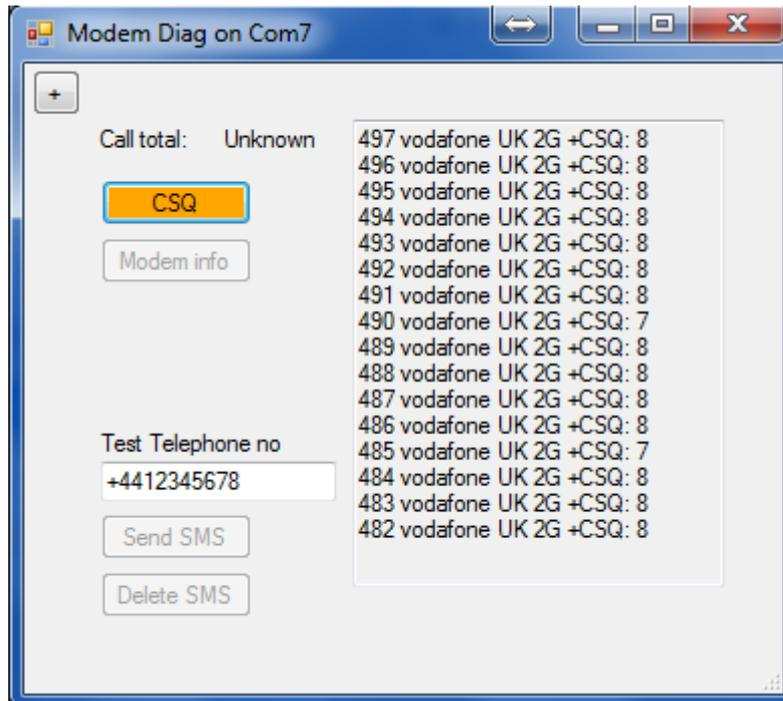
39) Click the 'CSQ' button; after a short period instantaneous signal levels will appear, this can be used to position your aerial in the best location to send data from CSQ ranges from 1 to 33. We always recommend CSQ be at least 7 or above for a chance of communication. To stop the test click the 'CSQ' button again.
