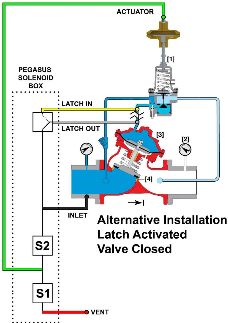
In the above alternative installation, the INLET and VENT connections are swapped around. When the Latch is activated, the upstream water is directly connected to the top chamber of the main valve [3], which fully closes the main valve. Due to the mechanical stops on the actuator, there will still be a small amount of flow through the pilot which enters as downstream water.
