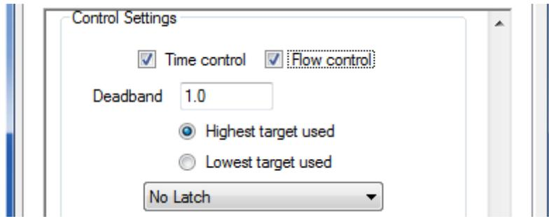
26) When selecting both time and flow control both sets of tables can be input as explained previously, however an extra option of either Highest or Lowest target used must be selected.
