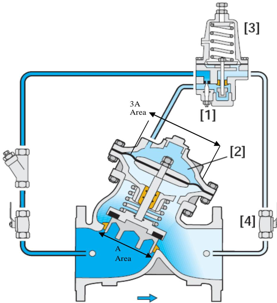
Opening process (Atmospheric chamber)
