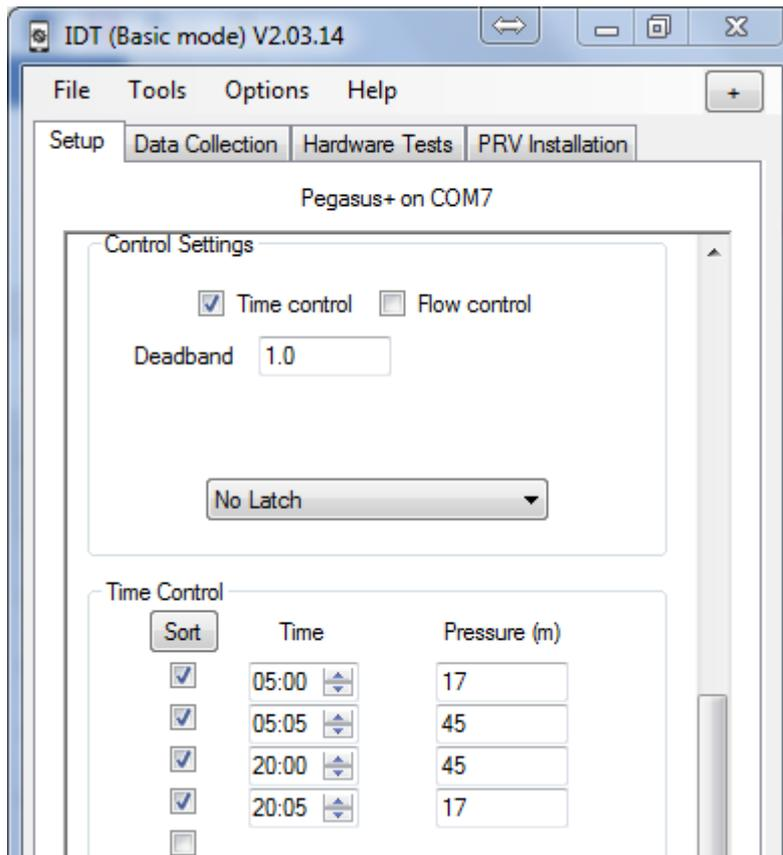
24) Enter times required, up to 32 entries can be used. Note the controller interpolates a diagonal straight line of pressure for the times between two points in the table.
