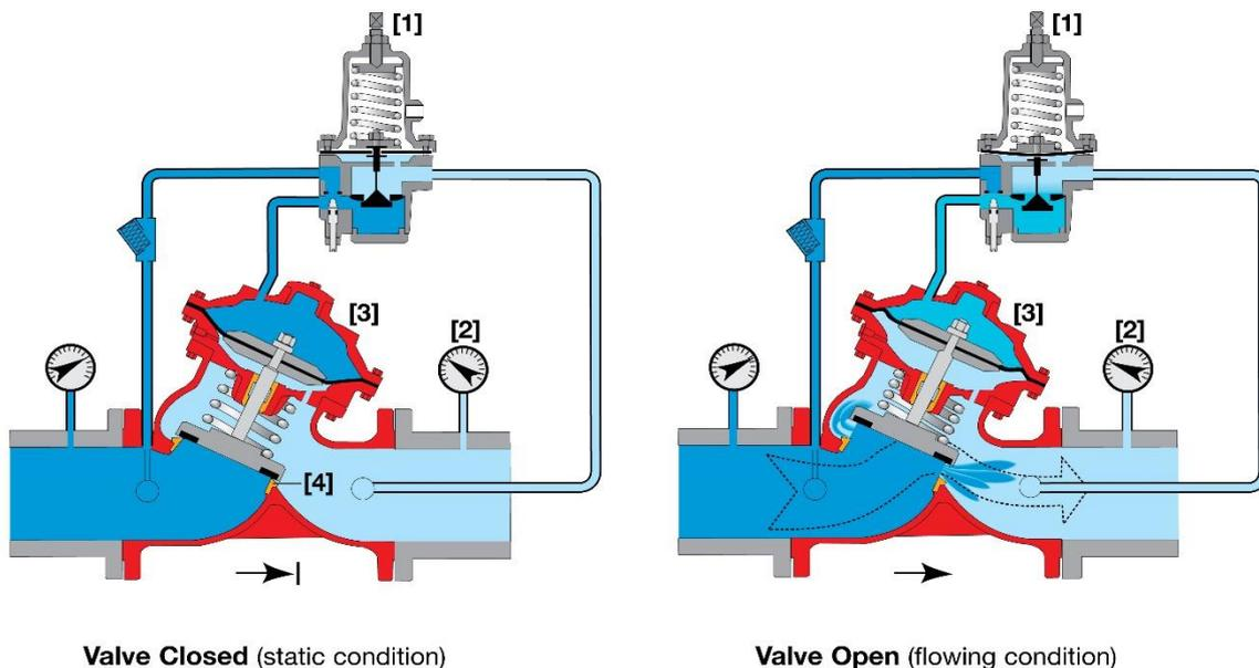
The HWM Pegasus Plus includes the HWM actuator which attaches to the top of the Pilot. This controls the pilot setting, and can be operated automatically and remotely, therefore controlling the downstream water pressure.
