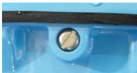
Figure 13: A photograph illustrating the pressure screw assembled
