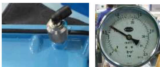
Figure 17: A photograph illustrating the test adaptor and a pressure gauge
