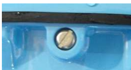
Figure 11: A photograph illustrating the pressure screw that needs to be removed and retained
