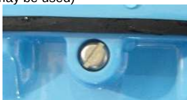
Figure 16: A photograph illustrating the pressure screw that needs to be removed and retained
