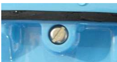
Figure 18: A photograph illustrating the pressure screw assembled
