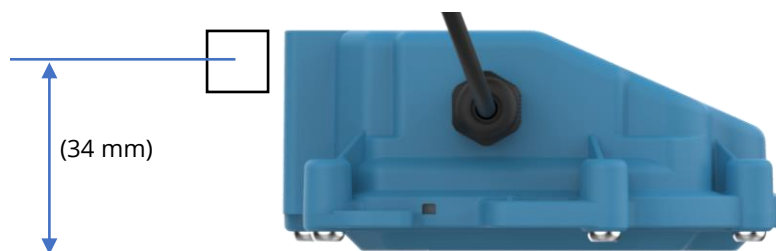
Figure 5. Offset (typical) of RadarSens from center of bracket arm (square)
