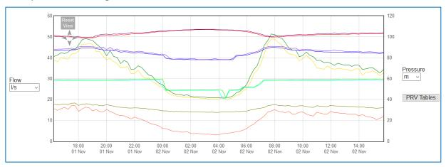
The PressView website allows the Sentinel 2 data to be combined with pressure measurements made (by another HWM logger device) some distance down-stream of the PRV (e.g. at a "critical point"). Both the local and remote measurements can be assessed by a user, and (whenever an adjustment is needed) revised pressure profiles can be sent to the Sentinel unit. This feature is not covered further in this document; refer to the User-Guide or instructions for PressView for more details.
