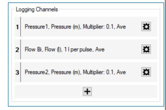
Channels can be added using the "+" button (e.g., if other optional interfaces are fitted).
