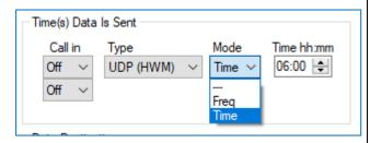
When Frequency is selected, it is not possible to add any additional lines to the table; just one exists.
