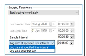
The "Sample Interval" is used to produce a set of data for the purpose of applying optional statistical functions (e.g. Average).
