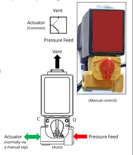
Adapters must be fitted onto the valve prior to connecting the hoses.
