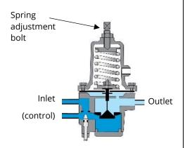
The water flowing into the pilot valve via the inlet port is restricted. This is typically done by a needle valve which may be either internal to the pilot valve or external to it (within the pipe feeding upstream water to the inlet of the pilot valve).
