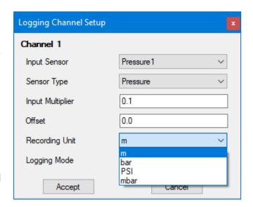
Or, put another way, the number obtained when the interface is read has to be multiplied by 0.1 to convert it to metres (m, the selected recording unit).
