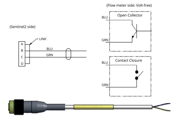
Connect the cable to the flow meter's volt-free pulse interface:
