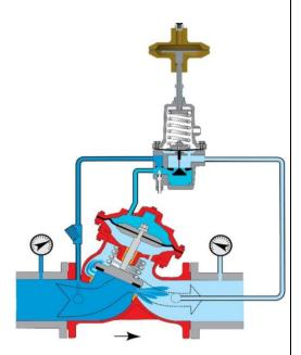
Whilst checking the outlet pressure of the PRV, **set the maximum pressure** required by adjusting the position of the **actuator bolt**.
