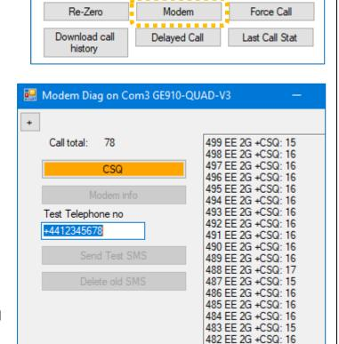
Move the antenna to various alternative locations to find the most suitable position. Stand well back from the antenna whilst the measurement is being made to ensure you are not blocking the signal.
