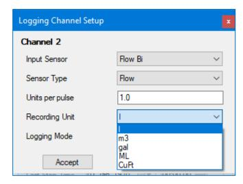
The appropriate scaling factor (Units per pulse) are also required. e.g. If 1 pulse represents 10 litres, "Units per pulse" should be set to "10".
