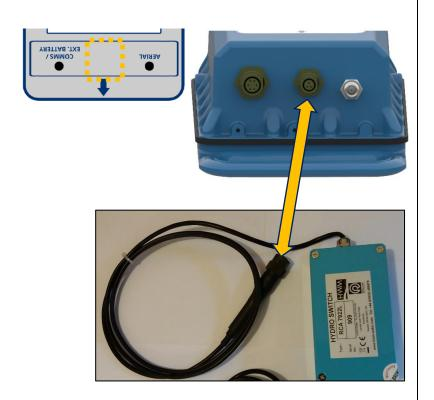
If required, the Hydroswitch can be tested prior to plumbing it into the system:
