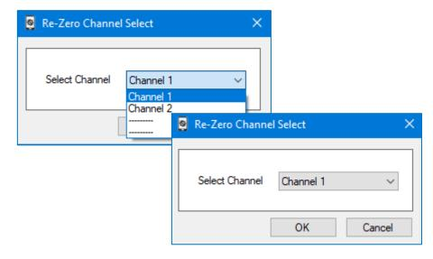
This starts the re-zeroing process of the Sentinel 2, which repeatedly reads the numeric output from the transducer.
