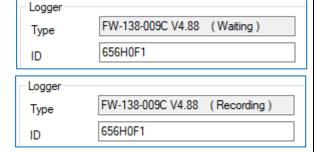
Note: The states for the built-in logger (Stopped, Waiting, Recording) have no effect on the PRV controller operation.
