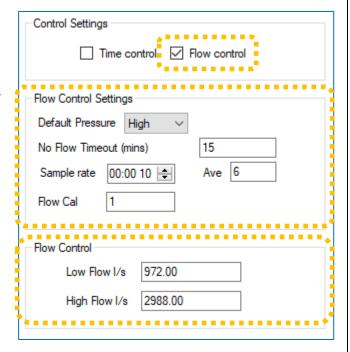
The general concept of Flow control is that Sentinel periodically makes an evaluation of the recent water demand to the downstream network and decides whether a High or Low pressure target is appropriate. It will then set the actuator to the required target pressure.
