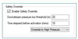
When enabled fill in the threshold settings and required action.
