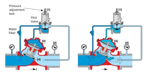
Valve Closed (static condition)
