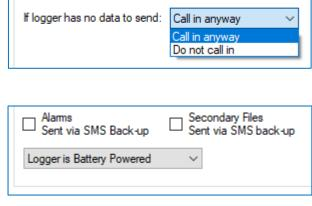
Tick the Alarms and Secondary Files (i.e. secondary data) if sending using the additional back-up method is also needed for these types of messages.
