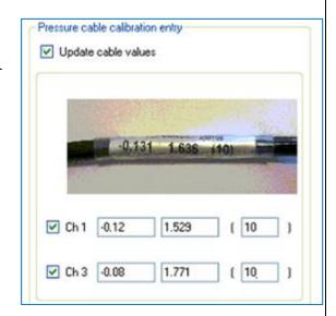
At this stage, it is important that the channel settings stored in the PC memory should be written into the Sentinel 2.
