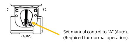
To change from "O" to "A", the manual override must be turned from "O" to "C" and then to "A" : "  $O \rightarrow C \rightarrow A$ ".
