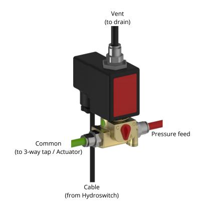
The Hydroswitch valve body is labelled (red and green dots) to assist in identifying the ports during installation.
