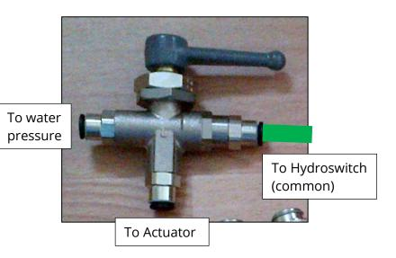
Fit adaptors as required to the 3-way valve of Hydroswitch.
