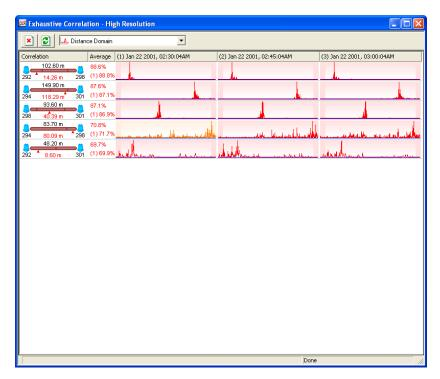
After correlation has finished the software sorts the data. The most likely leak correlations will be at the top.
