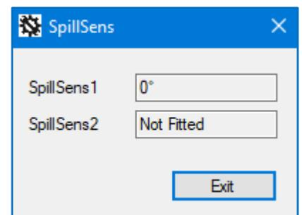
Tilt the sensor through various angles and observe that the angle changes; it is operating correctly.
