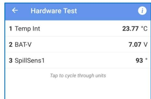
Position the sensor upright using a jig or alternatively disconnect SpillSens after completing the test. The SpillSens channel must be re-armed.
