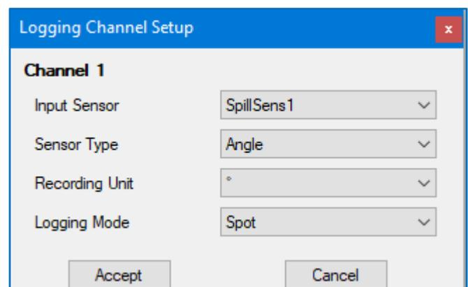
The Logging Channels panel now lists this channel along with a summary of the settings for interpreting the raw (numeric) data from this channel; it is to be interpreted as an angle measurement.
