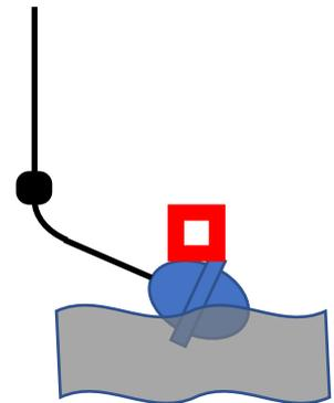
The SpillSens should also be positioned such that its cable cannot become entangled with any object during the rise and fall of water or due to turbulence.
