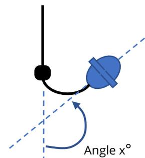
The *server* will typically regard the message of going above or below the threshold angle as the start of a meaningful event (i.e. a potential spillage warning), or the end of an event (problem over) respectively.
