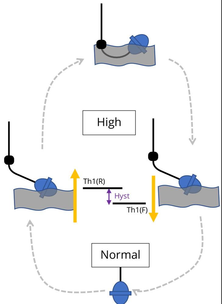
It should be noted that the above diagram illustrates the setup of a logger with a *single* trigger programmed into it, monitoring for SpillSens exceeding a specified angle. However, the logger can be programmed with *multiple* triggers, and thus it can monitor for SpillSens exceeding *multiple* angles.
