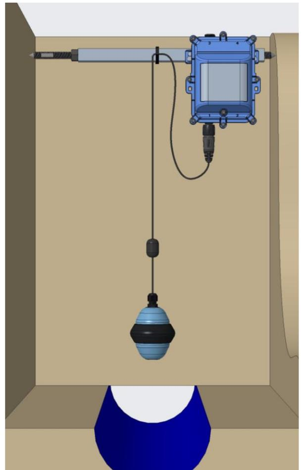
The SpillSens should be allowed to settle and come to rest. Once any swinging has stopped, **it must be connected to the logger** (see section 8).
