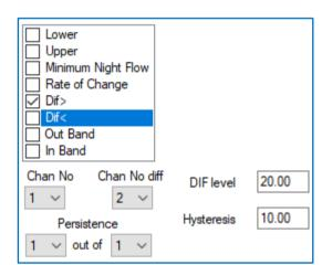
Similarly, an alarm set as shown opposite will compare the values of datapoints from the two selected channels (here, channel 1 and channel 2).
