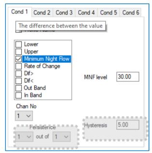
Note: Hysteresis settings have no bearing on the function of this trigger. Persistence settings have no bearing on the function of this trigger.
