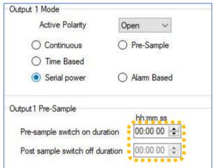
These settings will switch the output port ten seconds before the data is logged and it would be held for 5 seconds afterwards. Then it would return to its inactive state.
