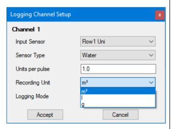
A relevant calibration factor for a water-meter is units per meter pulse. (Other types of equipment may require a different type of calibration factor).
