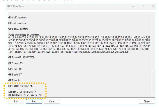
The window is a terminal which will display various messages as the test proceeds. The messages can be ignored, except for the ones which confirms that the logger has received an accurate time reference from the satellite, unless required for diagnostic purposes.
