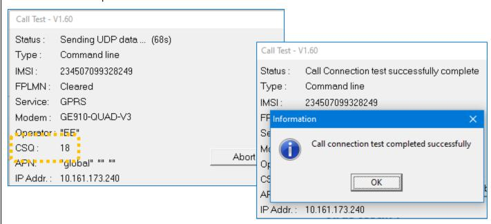
Confirm that a "Call connection test successfully complete" information box appears. Note the parameter "CSQ"; this is an important indication of the signal strength with the antenna in the current position.
