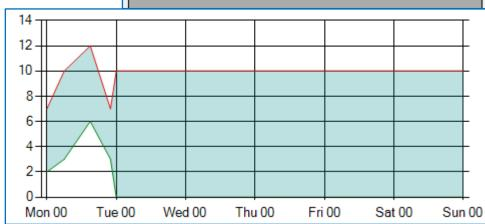
If a step change is needed, create additional lines within the table to ramp up or down to the new value in a short time, maybe a few seconds after the change is required.
