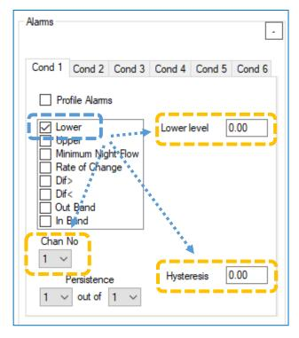
The relevant channel(s) have to be selected within the tab. The channels must have previously been set up and also saved to the logger; if not, they are unavailable for selection.
