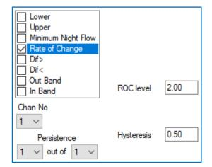
The Rate of Change trigger acts on datapoints which are increasing in value. (There is no equivalent trigger for datapoints that are decreasing in value).
