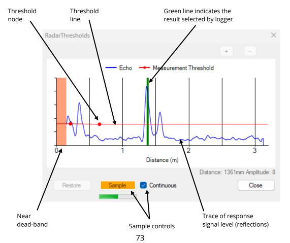
The RadarSens trace response shows the returned signal level, which comprises of a general noise-floor plus any signal peaks. The RadarSens has various strategies for selecting what it judges to be the correct peak for the water level. Generally, this will be the most dominant peak. However, it is possible that strong peaks of 'nuisance reflections' could also be present.
