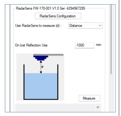
Sensor measurement issues (i.e., lost reflections) can be detected in the datapoint stream by setup of a 'lost reflection value' which is out of the range of normal data.
