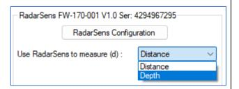
When Depth is selected, IDT requires additional information about the chamber and sensor position. Measure from the bottom of the chamber to the lower face of the installed RadarSens (re-check and adjust if the sensor position is ever adjusted).
