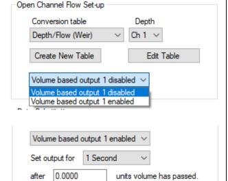
Set the required pulse duration and the number of units of volume required to pass to activate each pulse event.
