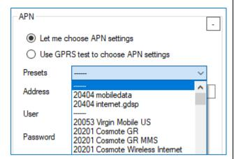
Alternatively, the user can enter the parameters for their fitted SIM card.
