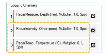
Depending on which channel you are currently setting up, select an Input Sensor of 'RadarIntensity' or 'RadarTemp'.
