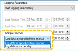
Most logger applications require the measurement interfaces to be logged frequently. For these, set to "Log data at specified time interval".
