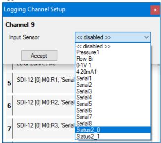
The "\_0" and "\_1" refers to the specific pin being used on the logger interface connector; refer to your logger user-guide for details of pin number or wire-colour of any HWM-supplied cable.
