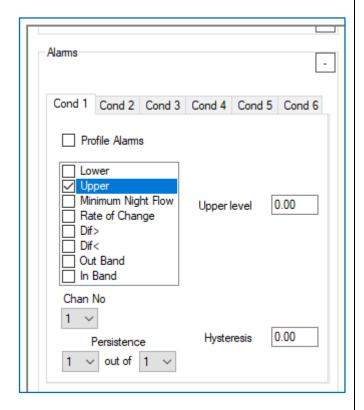
Set the Chan No to match the channel number for the sensor. (e.g. The SpillSens is located at channel "1", so set the Chan No to "1").
