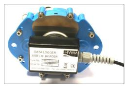
Connect the USB connector to the PC.
