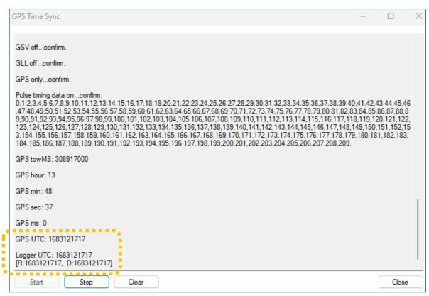
The window is a terminal which will display various messages as the test proceeds. The messages can be ignored, except for the ones which confirms that the logger has received an accurate time reference from the satellite, unless required for diagnostic purposes.
