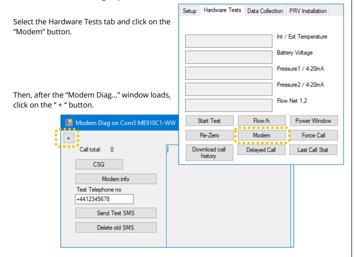
A unit with a 4G network capable modem will have an additional button, "Change Band / Technology" present.
