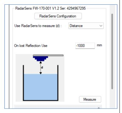
Next, set up the logger to handle the datapoint stream for situations where the RadarSens is unable to detect a reflection signal of any significance. These are known as 'lost reflections'. (Typically, this will be due to a sensor which has not been correctly tuned to the site, or if the channel is dry and unreflective).
