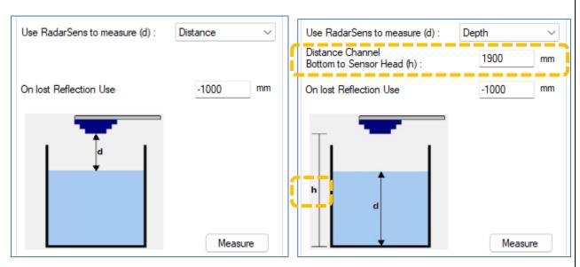
Note: The selected settings will not be saved to the logger using the normal 'Setup Device' button. Instead, you have to make a measurement using **the 'Measure' button**, as described below. **This saves the settings to both logger and the sensor.**
