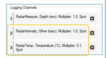
Depending on which channel you are currently setting up, select an Input Sensor of 'RadarIntensity' or 'RadarTemp'.
