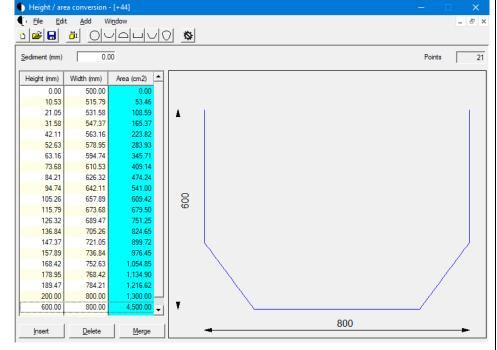
The cross-sectional area table must be saved to the logger using the "Transfer Data" button/icon.
