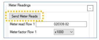
The current meter readings can be obtained by re-reading the logger; they will be displayed here.
