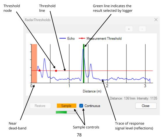
The RadarSens trace response shows the returned signal level, which comprises of a general noise-floor plus any signal peaks. The RadarSens has various strategies for selecting what it judges to be the correct peak for the water level. Generally, this will be the most dominant peak. However, it is possible that strong peaks of 'nuisance reflections' could also be present.
