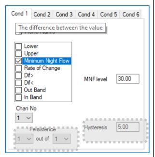
Note: Hysteresis settings have no bearing on the function of this trigger.
