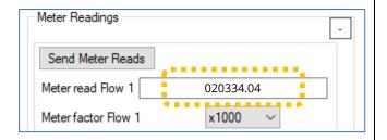
After waiting for the meter to change by a few digits, note the meter reading and re-read the logger to refresh the meter reading values held by IDT. Confirm the updated reading matches the actual meter reading (noted earlier).
