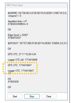
The messages may vary, depending on the GPS device fitted inside the logger and satellites found. Examples of the messages that indicate successful test completion ('GPS UTC: ...' and 'Logger UTC: ...') are shown above. When these are shown, click on the "Stop" button and close the GPS Time Sync window.
