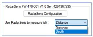
When Depth is selected, IDT requires additional information about the chamber and sensor position. Measure from the bottom of the water channel (or Riverbed, or the internal base of a fluid containment vessel) to the lower face of the installed RadarSens. (Re-check and adjust if the sensor position is ever adjusted).
