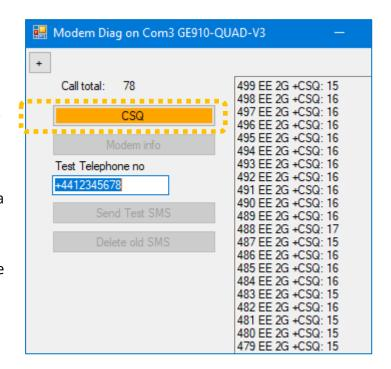
Initially, this test should be done with an open chamber. This is to verify that the connection to the mobile network works, and to determine what the local signal strength is.
