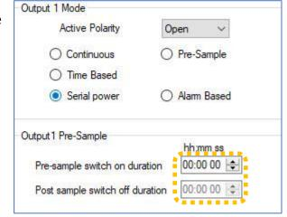
These settings will switch the output port ten seconds before the data is logged and it would be held for 5 seconds afterwards. Then it would return to its inactive state.
