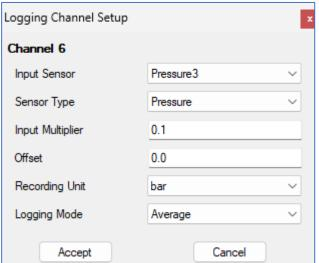
Setup of an external pressure sensor interface to record depth is similar. Select 'Depth' as the sensor type and then select a Recording Unit to the desired unit of measure (m, cm, mm ... etc).
