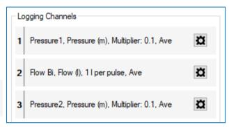
Note: Logger channels may be pre-configured by the factory prior to shipment, but the installer is responsible for confirming they are correctly configured to suit the installation site.
