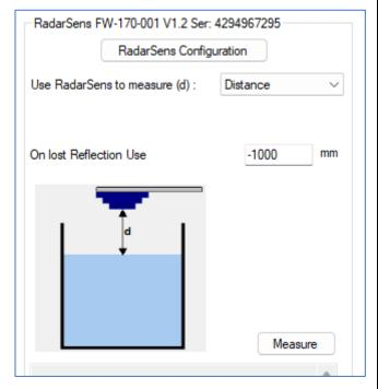
Next, set up the logger to handle the datapoint stream for situations where the RadarSens is unable to detect a reflection signal of any significance. These are known as 'lost reflections'. (Typically, this will be due to a sensor which has not been correctly tuned to the site, or if the channel is dry and unreflective).
