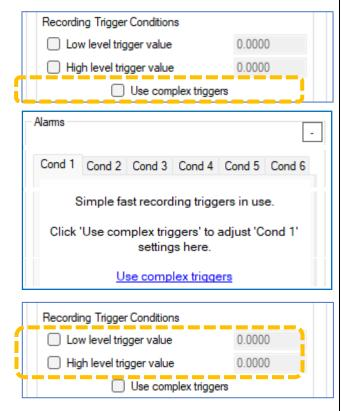
If simpler settings do not suit the application needs, enable the 'Use complex settings' to revert to normal setup.
