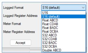
e.g., A velocity sensor manual says that the velocity (in m/s) is stored in address 1000 and uses a "Float 32" number format.
