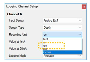
Adjust the 'Value at 4mA' and 'Value at 20mA' fields to the corresponding measurement values (using the recording unit of measure) that the sensor indicates at these current levels. (Refer to the sensor documentation).
