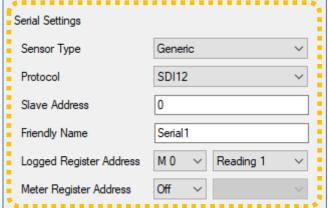
The sensor equipment may hold the data in one of several addressable registers; these will be sensor specific. Therefore, to access specific data from a sensor, both protocols will require the setup of accompanying parameters. (These are shown after the protocol has been selected).
