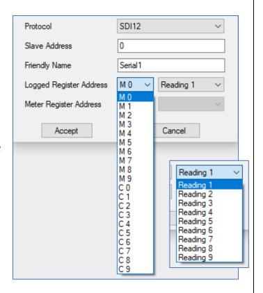
Where there are multiple sensor devices on the same SDI-12 bus, use the "C" command. ("C" is the concurrent command. Whilst waiting for one sensor, the logger can address other sensors on the bus; All must be accessed with the "C" command).
