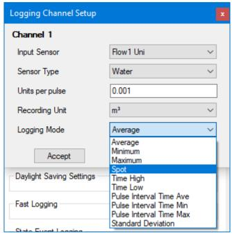
By repeatedly counting the number of pulses from the meter over a fixed period of time (the log period), the logger is able to determine the flow rate through the meter.
