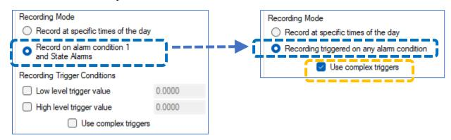
When 'Secondary recording' is set, setup is similar to 'Transient recording', except that the sensor input is less constrained. Because of this, the 'Trigger channel' control has to be set to identify the desired logger data channel number for which the simplified settings are applicable.
