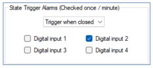
Note that the state switches are sampled *once per minute* regardless of the sample rate setting. If faster rates of state checking are required, the standard alarms should be used.
