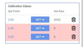
When the table is complete, tap on the save button to store the calibration table into the logger.
