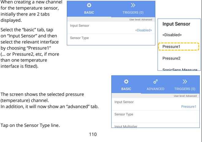
Sensor Type Then select the physical parameter of "Temperature" from the displayed list. Temperature Select the required **Recording Unit Recording Unit** recording unit and logging mode for Logging Mode °C Logging Mode Average producing the channel datapoints. °F Average (The recording unit Minimum selections listed are now appropriate to Maximum temperature measurement). Spot Standard Deviation
