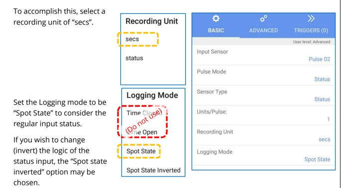
(e.g., This may be required for a switch which has a "normally closed" rather than a "normally open" condition).
