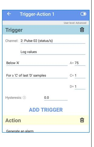
Setting A as "101" (or higher) will not permit the logger to clear from being triggered since the data value would always be below this; the data range for this channel data stream is always "100" (or below).
