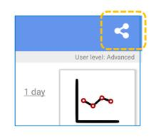
IDT offers the option of either copying the data to the clipboard (to be able to paste the data into another application), or to generate an e-mail with the data.
