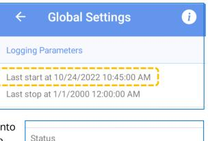
Note: A re-start of the logger deletes any previously stored data and begins storing fresh data. It is therefore important to retrieve any data from the logger prior to either stopping the logger or making any program changes.
