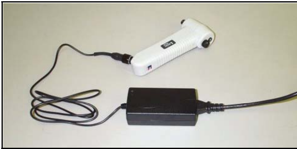
The Lmic connected to the universal 110-240V AC charger
