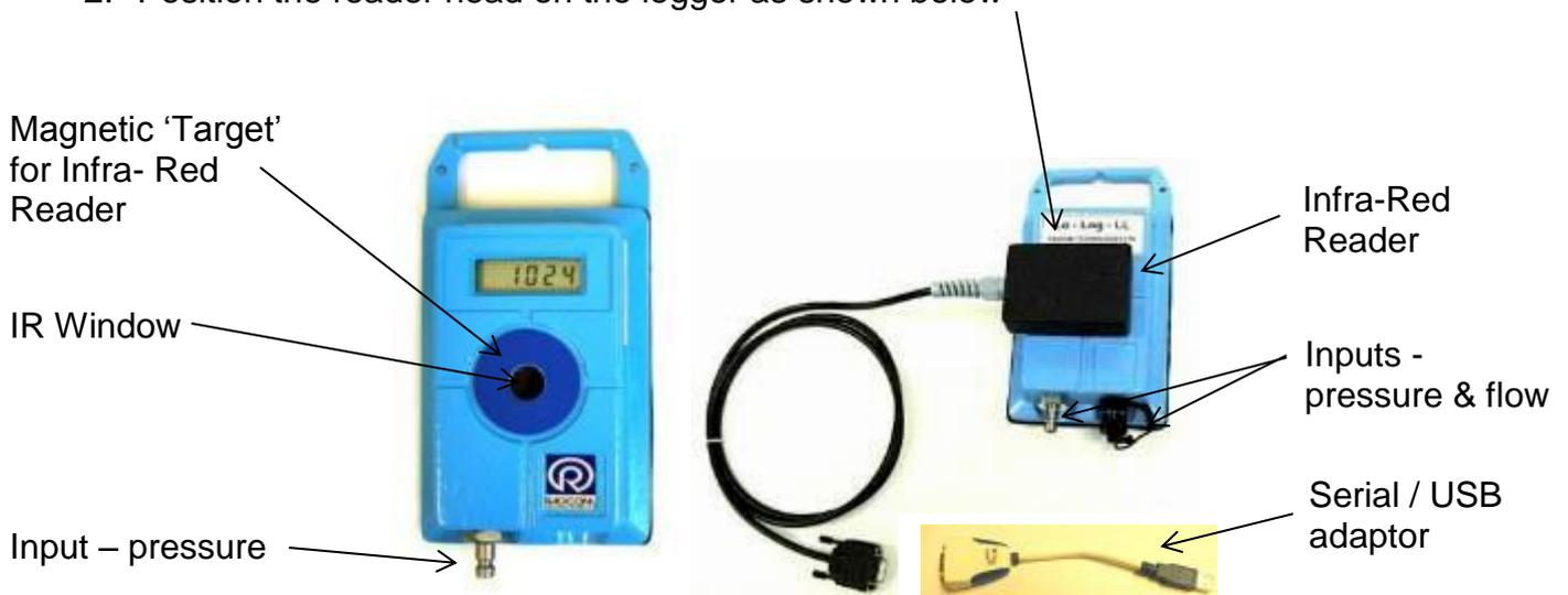
Take care to position the head over raised ring area around the window. The reader head will hold onto the logger by magnets in the ring around the window and this helps with positioning.
