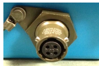
Figure 16. Flow sensor interface with a 4-pin MIL-spec connector
