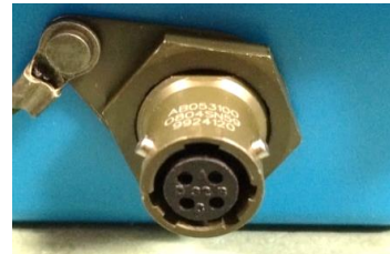
Figure 18. 4-20mA sensor interface with a 4-pin MIL-spec connector
