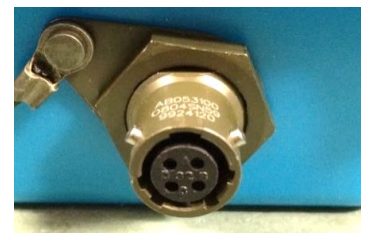
Figure 14. Pressure interface with a 4-pin MIL-spec connector
