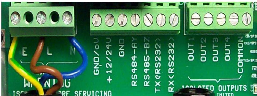
Data and power connections should always be made using screened cable. Using a screened cable will help to reject interference. You should always use a common ground point and avoid the formation of current loops.
