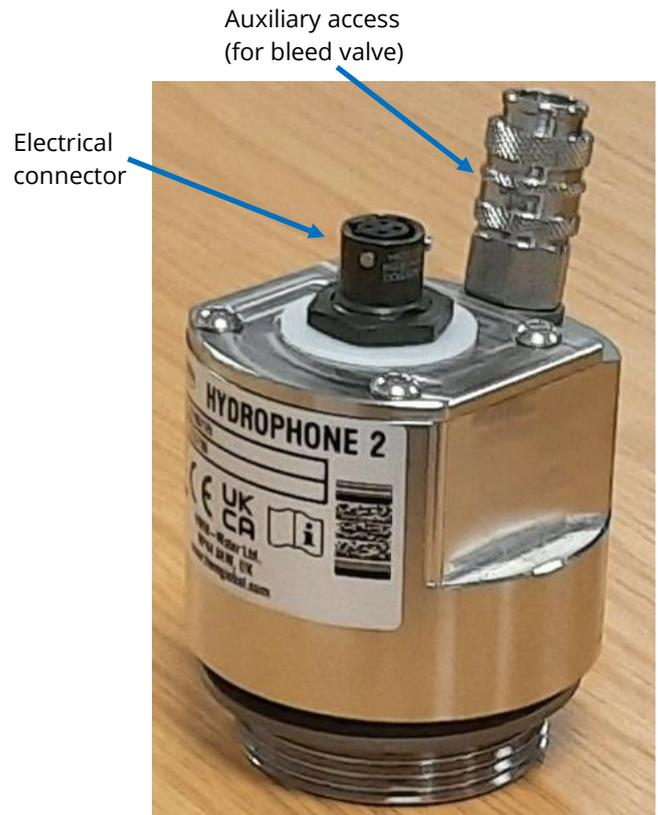
View showing cable and bleed-valve connections.
