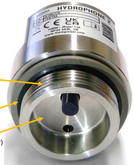
Various adaptors (options) can be fitted to the Hydrophone-2. Select a suitable one for use with the asset (valve, hydrant, etc) to which the Hydrophone is going to be connected.
