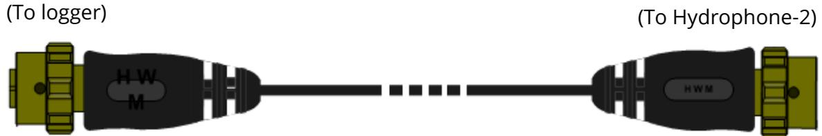
One connector has pins ; connect this to the Hydrophone 2, as shown opposite.
