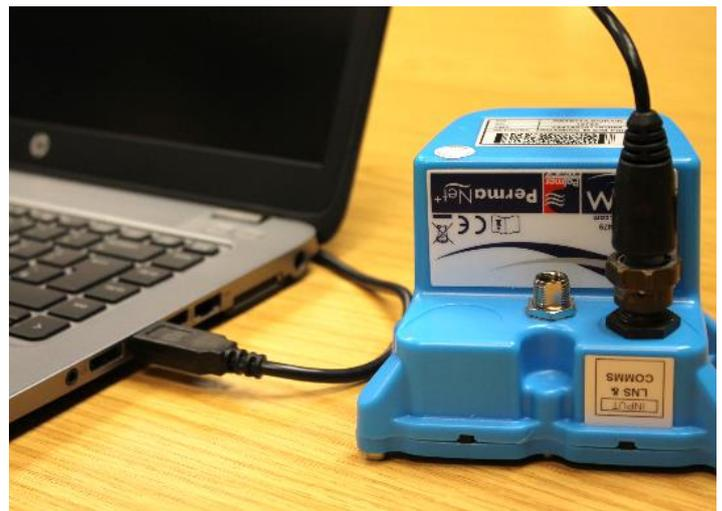
Note: The first time you connect your PermaNet+ to a new USB port, Windows will configure the driver; Wait until this process is completed before proceeding.
