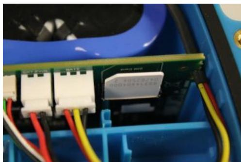
3. Insert your new SIM into the empty slot as shown above. Ensure the gold contacts face the board and the notch is to the left.
