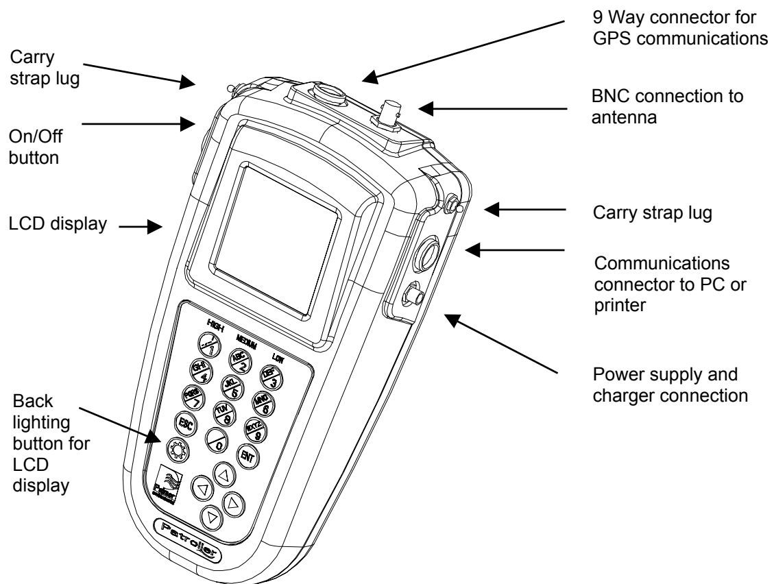
Patroller unit: connections and interfaces
